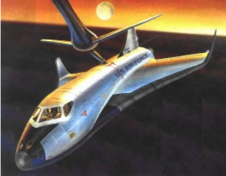
Fig 3. Black Horse Rocketplane Design—all-rocket propulsion
